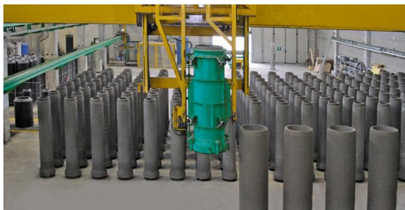
Figure 3-4: Concrete pipe manufacturing, Jaipur (photo: Yash Raj)
