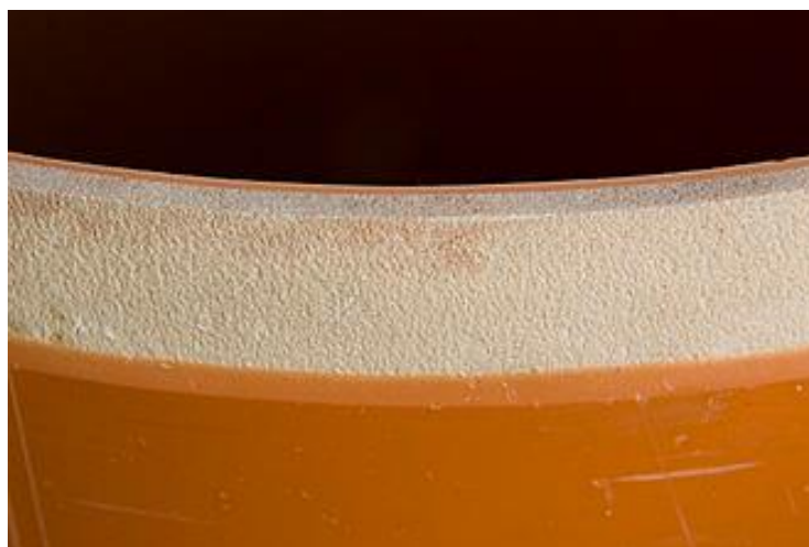
Figure 3-1: PVC-Pipe with foamed core
