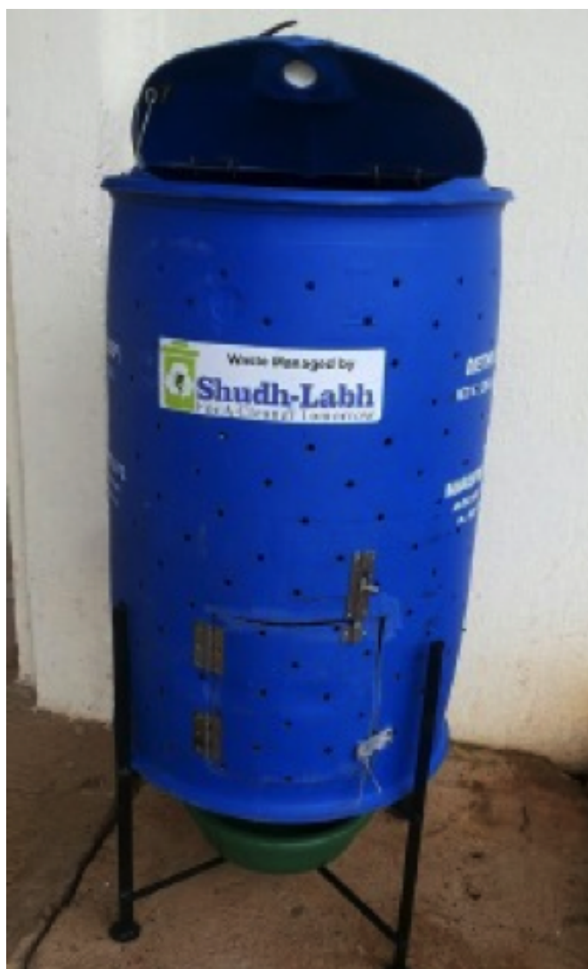
Blue HDPE Compost Digester
